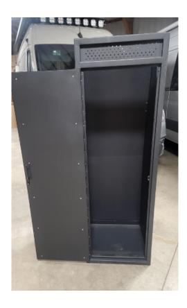
From this step, slide the shower into its final location. This is a good time to think about final drain placement and wiring for any lights above the shower. Once the drain is set, the shower stall can be secured to the van.
